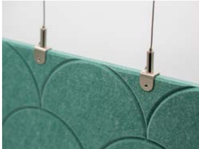
Anchor C to hang 9-12 mm thickness suspended panel with steel cable. Adjusted included (from 150 mm to 2000 mm).
